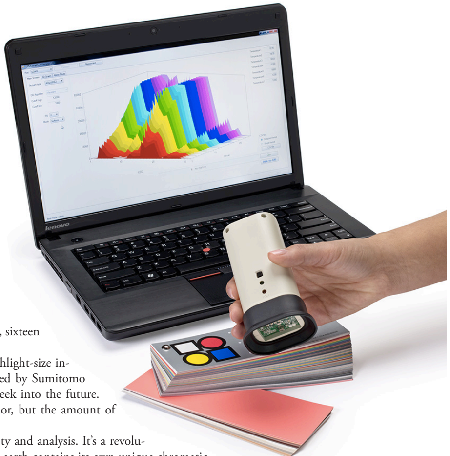
THE HANDHELD CYCLOPS device uses Visualant's patented ChromaID technology.
